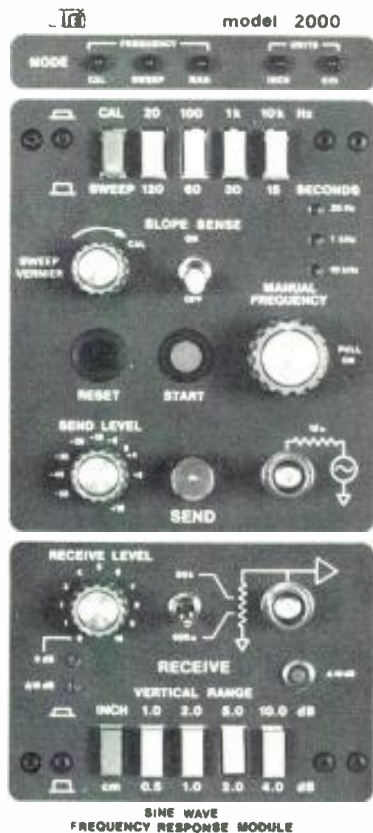
Figure 1. The face of the Model 2000 plug in module. The apparent knob directly below the word send at the center of the unit is actually a knurled screw that secures the module into the frame.
